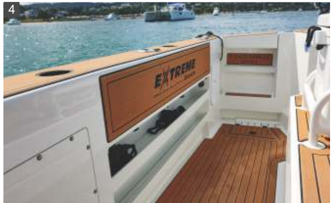
1) Tackle can be left on board with the knowledge it will be safe in a lock-up cabin. 2) The two large drawers under the helm station are ideal for tackle storage. 3) The helm station is dominated by a 22" Garmin screen. 4) More SeaDek provides waist height padding for anglers tackling a decent fish. A transom door makes bringing the bigger fish on board an easier task.
