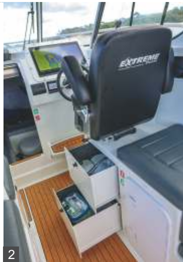
1) Tackle can be left on board with the knowledge it will be safe in a lock-up cabin. 2) The two large drawers under the helm station are ideal for tackle storage. 3) The helm station is dominated by a 22" Garmin screen. 4) More SeaDek provides waist height padding for anglers tackling a decent fish. A transom door makes bringing the bigger fish on board an easier task.
