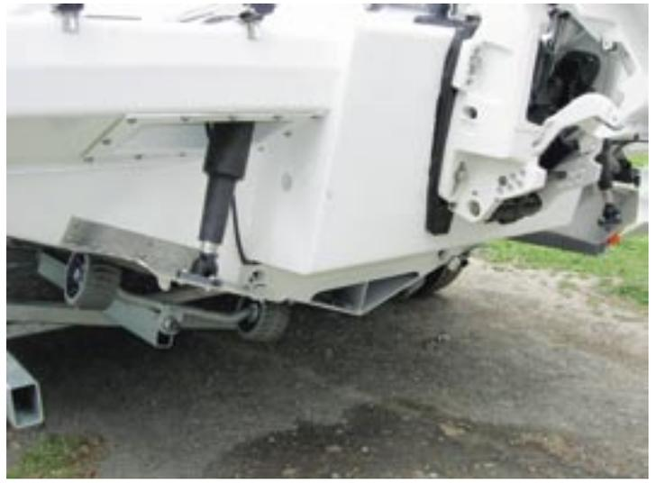
Trim tabs have off-hull mounts, avoiding the need to drill mounting holes in the hull.
