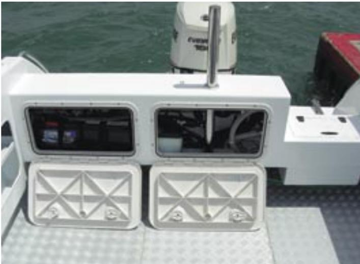
*Transom lockers store the batteries in a protected position*
