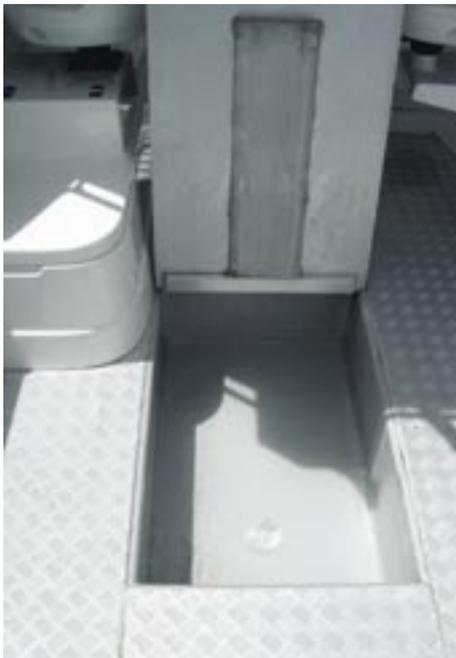
Central under deck holds can be flooded by removing a bung.
