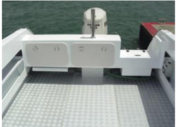
*The chequerplate decking extends right to the sides, providing good footing.*
